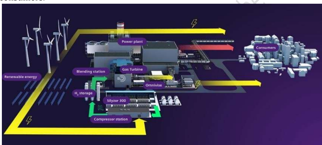
Fig. 3.16: Green Hydrogen production plant and gas power plant with hydrogen storage
