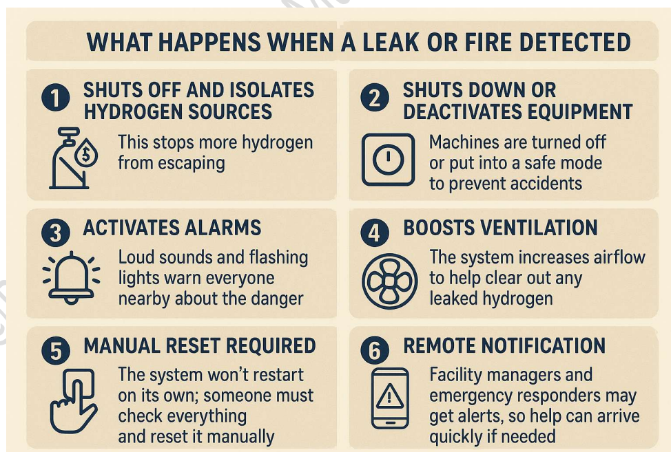
Fig 5.16: Control System after a Hydrogen Leak or Fire is Detected
